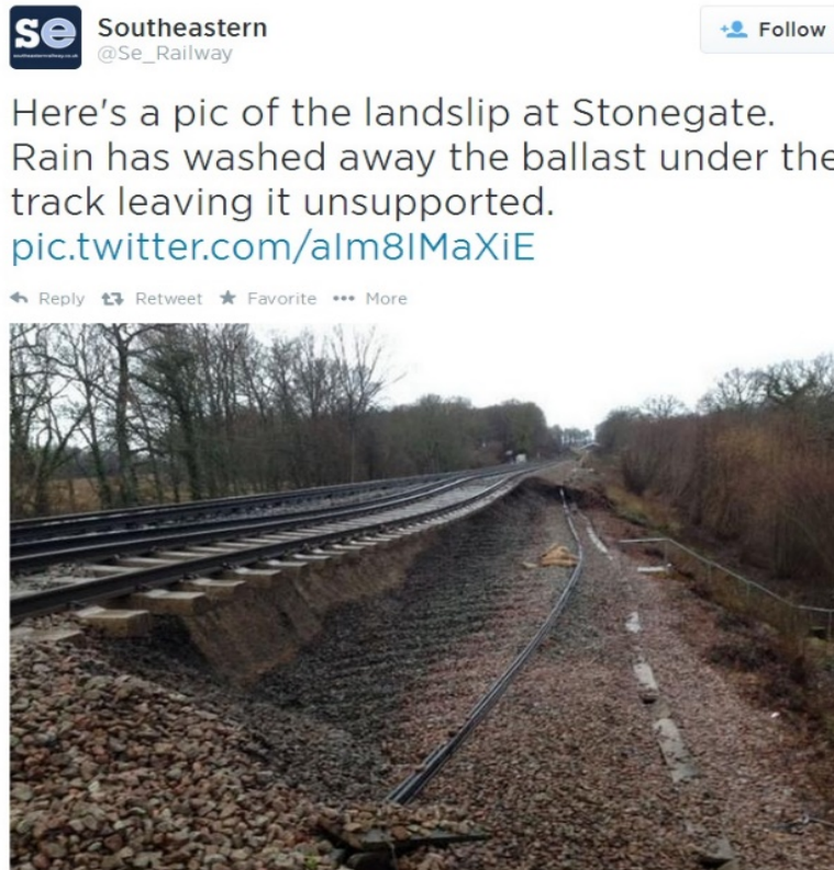
One of rail operator Southeastern's tweets about the line closure at Stonegate showing a picture of the problem
