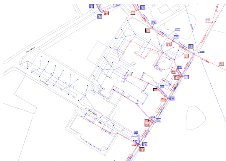
FIGURE 2 EXAMPLE SEWER NETWORK PLAN MAP USED IN BUILDING THE MIKE URBAN MODEL.
